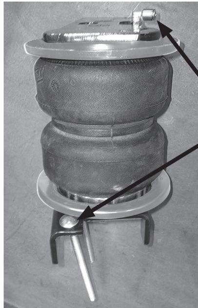
Attach the lower brackets so the carriage bolts are opposite of the fitting on the air spring assembly.
