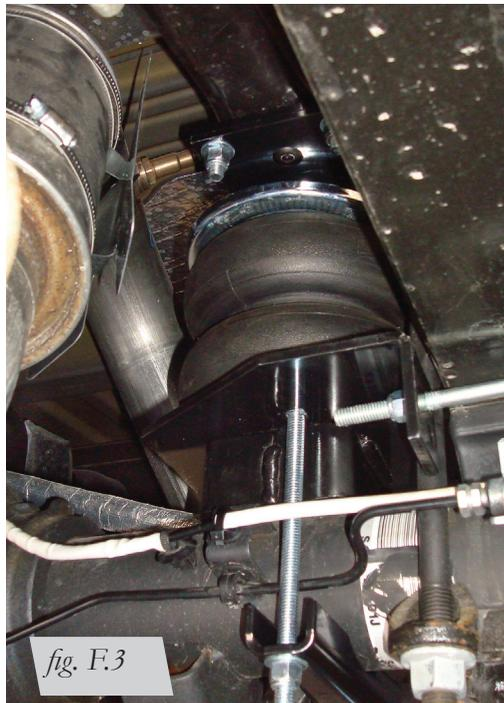
Passenger's (right) side rear view of kit installed.
