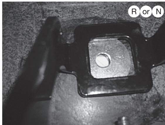
For the passenger's side, before inserting the upper brace hardware, make sure that the 1/2" thick washer (R) or (N) is installed in between the brace and frame (see Step 2). Note: The 1/2" thick washer (R) is not a half inch thick. It has a 1/2" hole and is a thick washer.
