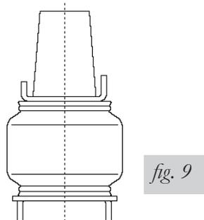
7. Tighten the upper bracket mounting hardware to 16 lb.-ft.
