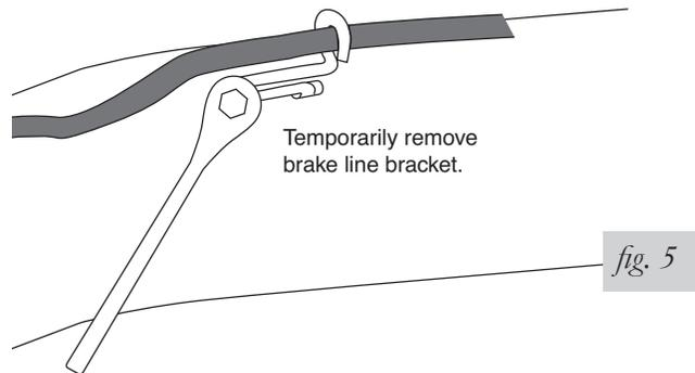
3. Lower the suspension so that clearance is provided to install the air spring unit. Do this by lowering the axle or raising the frame.
