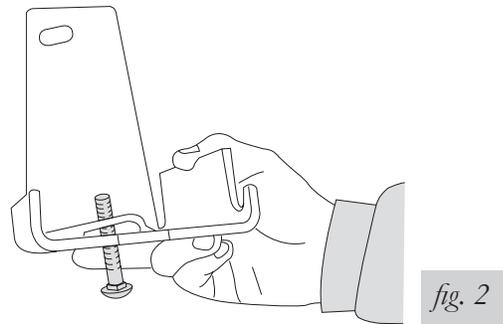
3. Set bracket and carriage bolt assembly on top of the bellow. Attach with two bolts (F) and lock washers (L).
