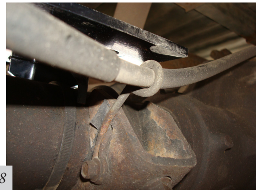
Bend wire bracket forward and down to clear bracket
