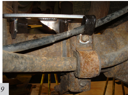
Attach frame clamp using new flange bolt, bend slightly
