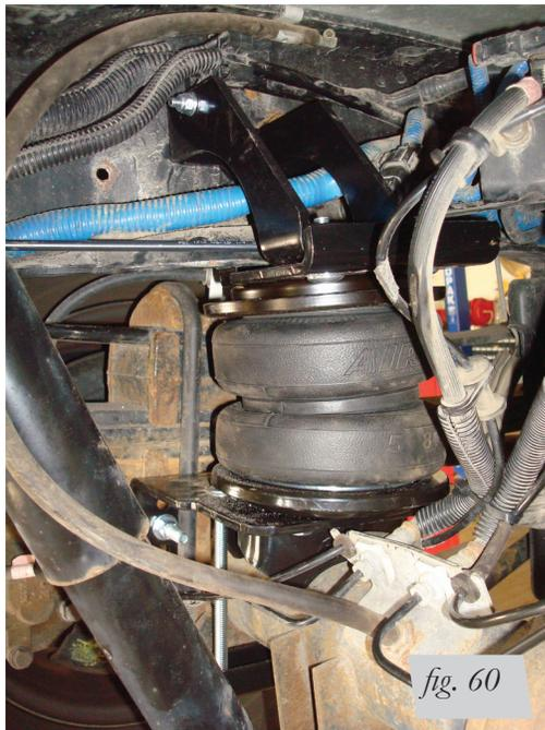
Driver's (left) side view of the kit installed from rear center of vehicle.
