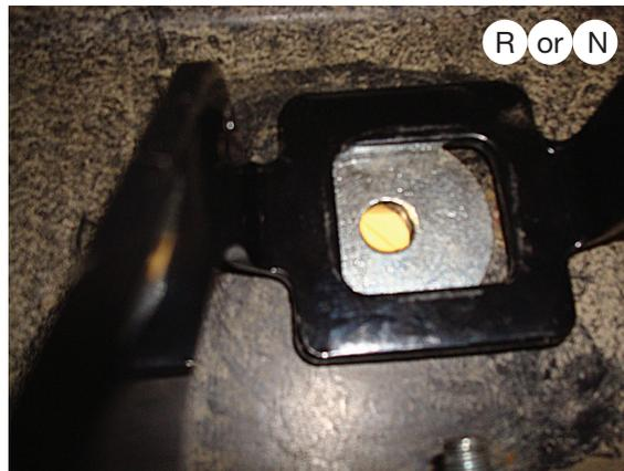
For the passenger's (right) side, before inserting the upper brace hardware, make sure that the 1/2" thick washer (R) or (N) is installed in between the brace and frame (see Step 2). Note: The 1/2" thick washer (R) is not a half inch thick. It has a 1/2" hole and is a thick washer.
