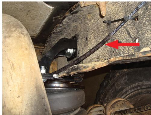
Air line thermal sleeve shown in place on the right side (passenger) of the vehicle. Make sure thermal sleeve is pushed up against the fitting once the air line is installed.
