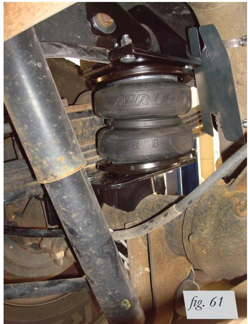
Passenger's (right) side view of the kit installed from forward of the axle.
