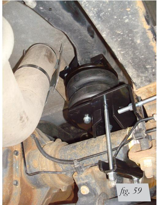
Passenger's (right) side view of the kit installed.
