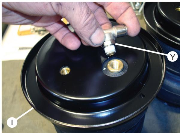
Set roll plate (I) over the air spring and install the fitting (Y) as stated. Repeat for both air springs.
