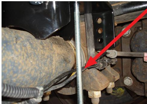
The long carriage bolt goes on the outside (backside) of the hard brake/ABS line on the passenger's (right) side.
