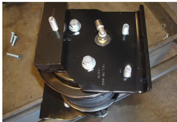
Spacer (H) set on bracket in position. The wide side of the spacer faces the outside of the vehicle.
