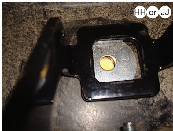
For the passenger's side, before inserting the upper brace hardware, make sure that the 1/2" thick washer (HH) or 3/4" washer (JJ) is installed in between the brace and frame (see Step 2). Note: The 1/2" thick washer (HH) is not a half inch thick. It has a 1/2" hole and is a thick washer.
