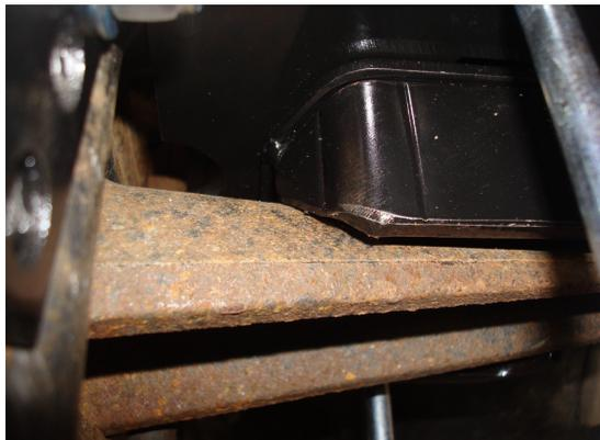
Make sure the cup is seated onto the jounce bumper strike plate forward and behind the axle.
