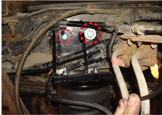
Tighten the M8 hardware and the **1/2" (or 3/4")** if from the 5th wheel hitch hardware) and tighten securely. Repeat for the hardware on the opposite side.
