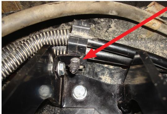
Insert the line holder previously removed into the L-bracket installed on the upper brace as shown.
