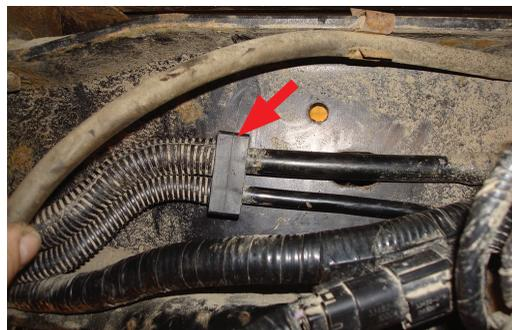
If equipped, this emissions/fuel line holder must be pulled away from the frame in order to install the upper frame brace (E).
