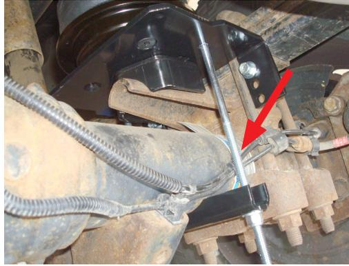
It may be necessary on some models to not tighten the axle clamp bar evenly on the right side (passenger's side) so that the clamp bar will clear the hard brake line.
