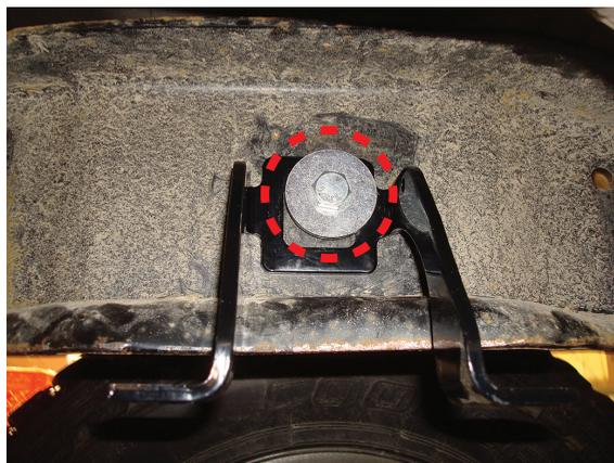
Passenger's side upper brace shown with hardware supplied in place.
