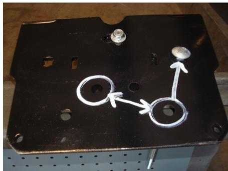
Passenger's side air spring mounting holes shown in location to the 3/8"-16 x 10" carriage bolt previously installed. When installing on the air spring, make sure the bracket edge facing you is on the fitting side of the air spring.
