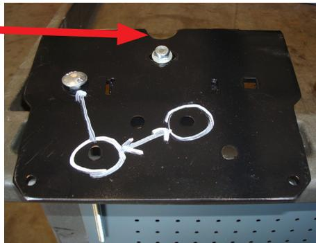
Driver's side air spring mounting holes shown in location to the 3/8"-16 x 10" carriage bolt previously installed. When installing on the air spring, make sure the bracket edge facing you is on the fitting side of the air spring.
