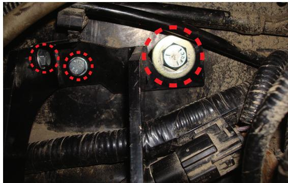
Driver's side brace shown with supplied hardware in place. Existing fifth wheel hardware which may have been removed may look different.
