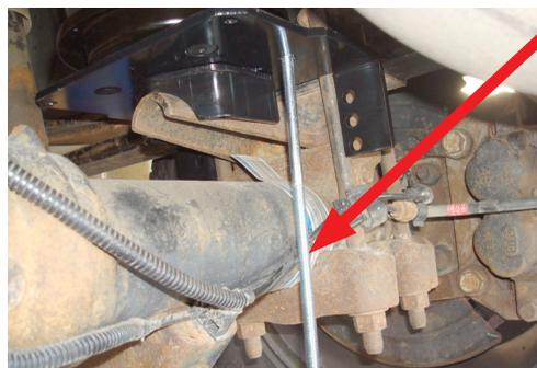
The long carriage bolt goes on the outside (backside) of the hard brake/ABS line on the passenger's side.
