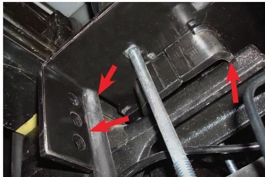
2. Install the U-bolts (H) around the jounce bumper strike plate/spacer blocks and insert through the topmost holes in the lower bracket main plates (Fig. D.16). Cap with the 3/8" flat washers (N) and 3/8"-16 nylon lock nuts (M). Snug bolts evenly, just enough to hold the lower bracket main plate flush against the stock U-bolts.
