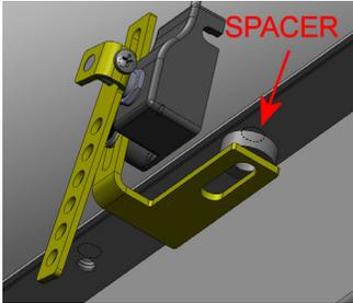
A close-up 3D diagram showing the yellow bracket being secured to a metal flange. A red arrow points to a small grey spacer between the bracket and the flange. The word "SPACER" is written in red above the arrow. |
