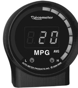
You can select the target fuel economy (MPG) for your vehicle by pressing and holding the right (data input) button while in instantaneous MPG mode. The display will show a target MPG which will increase from 5 to 50 in increments of 5 MPG. Continue to press the right button until your target MPG is displayed, then release. This target MPG will then translate to an ecograph with the top green LED illuminated.
