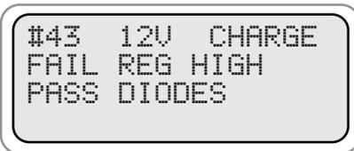
High Regulation will damage the system. Replace or repair the Alternator.
