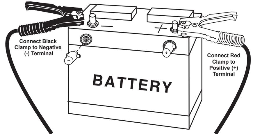
**Note!** Take special care when connecting to battery side terminals. If necessary use a side post adapter to prevent thread damage. When testing dual post batteries always check the post to which the system is attached. If a load test is made from a post connection and the alternator is mounted to side terminals a battery load test can be completed, but a continuity problem may still be in the side terminals when testing the alternator.
