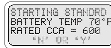
Confirm that the inputs are correct. Press "Y" is they are correct. The test will start. Press "N" to re-enter battery type, temp, and rating.
