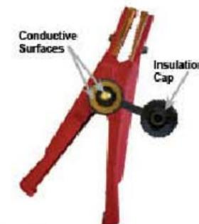
**WARNING!** insulation cap must be installed (on red clamp) when performing in vehicle test to prevent potential arcing.
