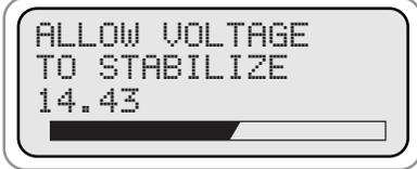
The BVA-350 will allow the voltage to stabilize before starting the test bar at the bottom of the screen that shows the test progress. Be patient, it can take up to 30 seconds for the voltage to stabilize.
