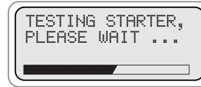
The BVA-350 will test the starting system. A bar at the bottom of the screen will show the tests progress.
