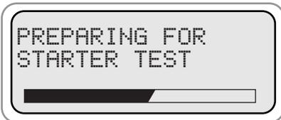
Press (Y) and tester prepares for the starter test. Bar at the bottom of the screen will show the progress.
