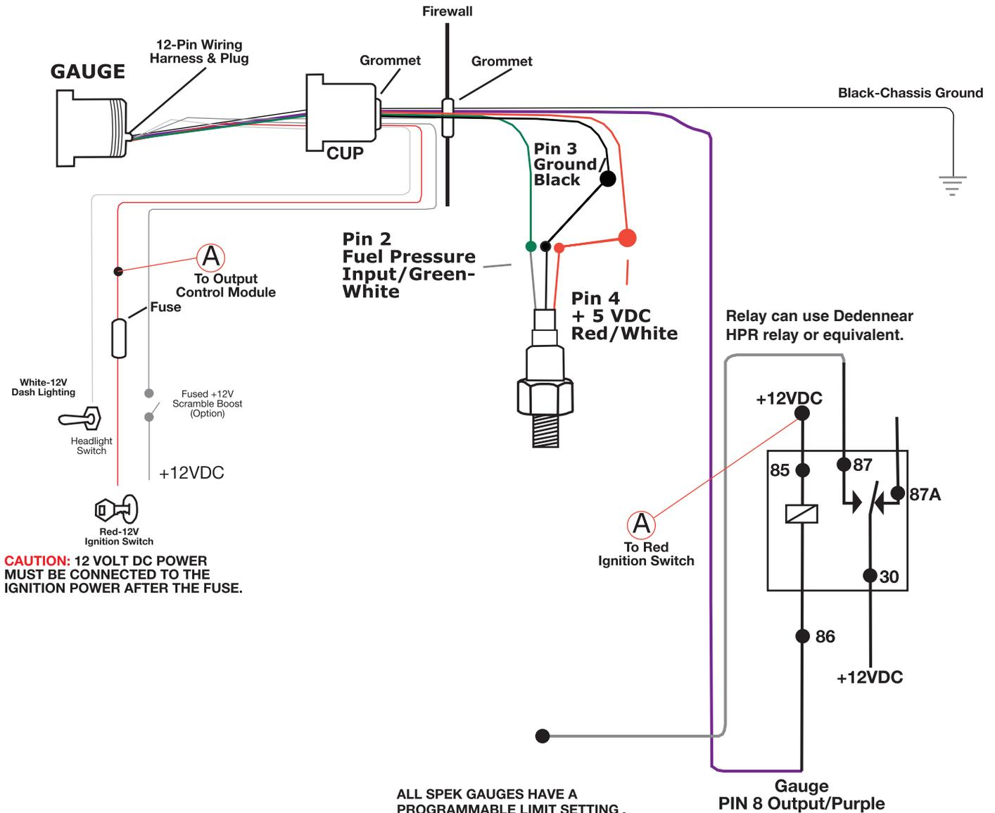
**CAUTION:** 12 VOLT DC POWER MUST BE CONNECTED TO THE IGNITION POWER AFTER THE FUSE.
