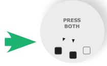
**Calibrate Gauge to Environment:** Turn the ignition ON with the engine OFF. While in the Normal Mode, press and hold the CENTER and LEFT buttons for five (5) seconds. The dial face plate will flash GREEN rapidly. Press the CENTER mode button to save the setting and return to NORMAL OPERATION.
