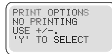
If the XCPRO-80 is connected to a POSI-160 interface that has a printer, you may chose "PRINT TO POSI" to be prompted to print the charge results.
