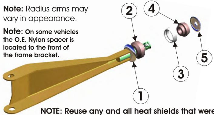
**NOTE:** Reuse any and all heat shields that were installed to protect the rear bushings.
