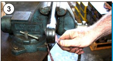
Remove any burrs and sharp edges with a file and emery paper as preparation for the new bushing. You want the edges smooth and rounded to ease installation and prevent cutting the bushing.
