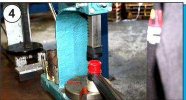
Grease inside of track rod and the leading edge of bushing. Press new bushing into the eye. (It may take multiple attempts, as bushing tends to bulge out a lot when compressed. It wont be easy, but it will go in).
