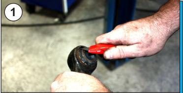
Factory outer metal shell must be pressed out. Use a razor knife to remove any excess rubber bushing. This will help prevent any binding while pressing out the bushing.
