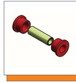
**Note:** Remove old bushings, clean ID of the control arm eyes. Apply a light coat of "Formula 5" grease to I.D, O.D. and Flange of the bushing. Apply a light coat of grease to the OD of the sleeve. Reassemble the bolt and torque to factory specs.
