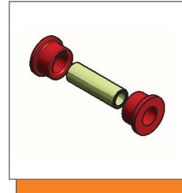
**Note:** Remove old bushings, clean ID of the control arm eyes. Apply a light coat of "Formula 5" grease to I.D, O.D. and Flange of the bushing. Apply a light coat of grease to the OD of the sleeve. Reassemble the bolt and torque to factory specs.
