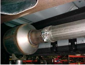
Lay out the exhaust on the floor so it looks like the drawing and compare parts with manual. To remove the stock exhaust remove it from the clamp located just behind the catalytic converter. Cut off your stock tailpipe for easier removal. Leave all rubber grommets in place. Use WD-40 to aid in removal of exhaust and hangers.
