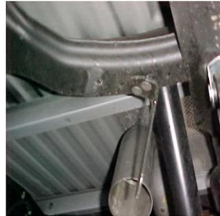
Next, remove spare tire. On pass. side there is a bracket that holds the spare tire in place. Remove it and spin it around 180 degrees. Now, re-install your spare tire.
