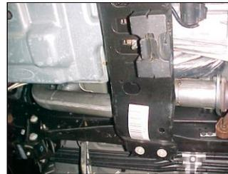
**5.** Install downpipe #K onto downpipe #J and secure with clamp #H. **DO NOT TIGHTEN.**
