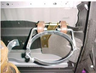
**3.** Install band clamp #F into rubber grommets located above the axle and attach bolt kit #I. DO NOT TIGHTEN.
