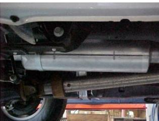
**4.** Install muffler #B onto headpipe 1½-2" with the louvers facing the converter. Secure with clamp #G. DO NOT TIGHTEN. Use a jack stand to support the muffler.
