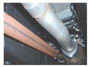
4. Install headpipe #A onto your existing stock front pipe Re-using the factory nuts.
