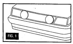
**CAUTION:** Make sure auxiliary lamps do not restrict airflow to the radiator or obstruct headlamps, turn signals or marker lamps.
