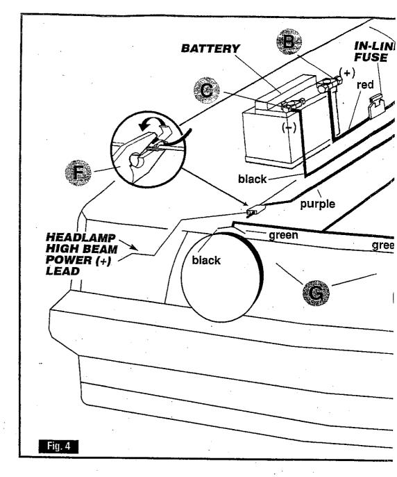
**b.** Connect ground wire (black) to ground or to the negative (-) battery terminal. (See C in Fig. 4) Use screw (provided) if necessary.
