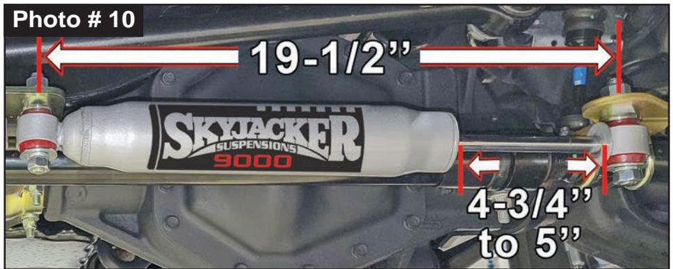
12. Cycle steering from side to side & check for adequate clearance. Check all brackets & bolts for proper installation.
