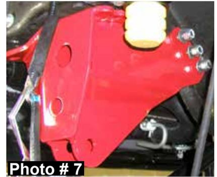
14. Attach the new Skyjacker track bar bracket to the frame using the OEM hardware.
