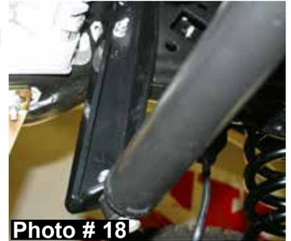
26. Install the new Skyjacker front shocks & lower the front of the vehicle to the ground.
