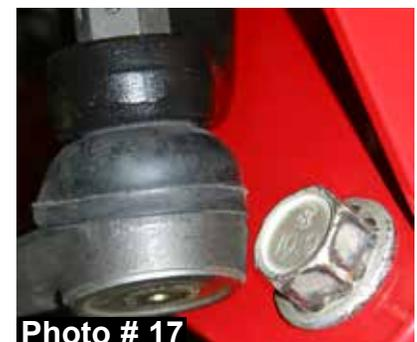
25. Attach the new Skyjacker steering stabilizer bracket to the frame by aligning the upper mounting hole of the bracket with the upper OEM stud on the frame & tighten using the OEM hardware. Attach the OEM stabilizer to the new bracket using the supplied 12mm nut. (See Photo # 18)
