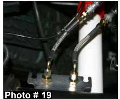
29. Disconnect the OEM rear brake lines & attach the new Skyjacker brake line extensions to the OEM brake lines. Attach the new Skyjacker brake line extensions to the OEM bracket using the OEM hardware & supplied plastic ties. (See Photo # 19)
