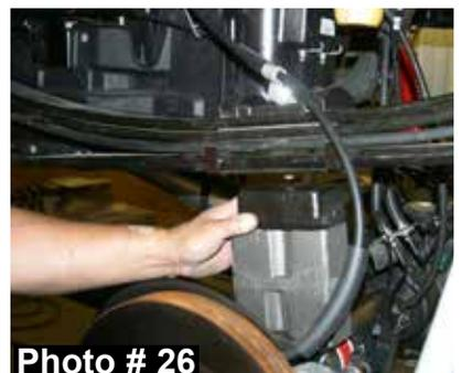
36. Install the new Skyjacker rear lift blocks with the taller end toward the rear bumper, between the axle pad & the OEM blocks **Note:** The new blocks will be installed below the OEM blocks. (See Photo # 26)
