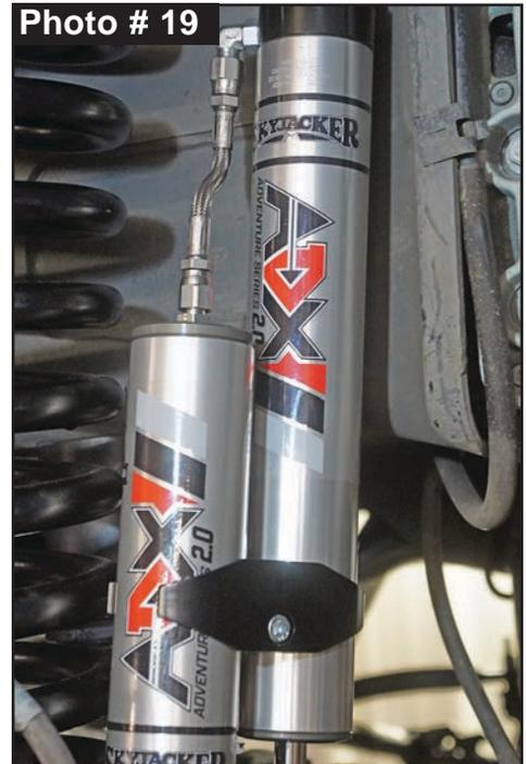
21. Connect Skyjacker front shock at upper shock tower mount using a 18mm socket \ wrench.
