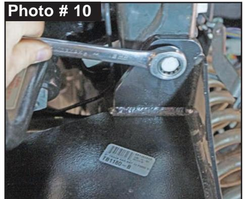
11. Remove OEM bump stop using adjustable channel lock pliers or a flat screwdriver.
