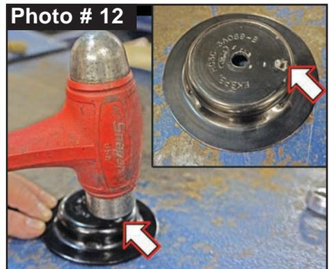
12. Place supplied 5/16" SAE Washer onto 8mm x 90mm bolt. Apply a few drops of supplied # LT100 Thread Lock Compound onto 8mm x 90mm bolt. Install Skyjacker # BSS275-B Bump Stop Spacer with OEM bump stop cup to the frame mount using a 13mm socket \ wrench. (Photo # 13)
