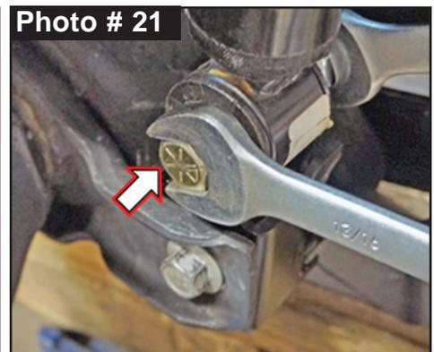
23. **Note:** Skyjacker Brake Line Extension Brackets Are Side Specific. # F23BE-D Driver & # F23BE-P Passenger.
