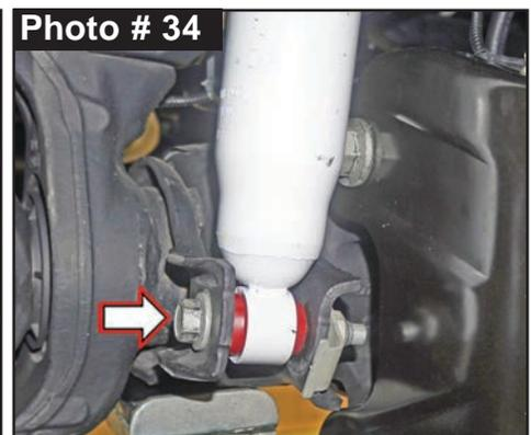
27. Locate Skyjacker ADX front shock. Loosely assemble two (2) supplied reservoir clamps with two (2) supplied hex head bolts using a hex key socket (one (1) front & one (1) back). Position clamp into place around shock body & reservoir cylinder. Secure, but **Do Not Completely Tighten**.
