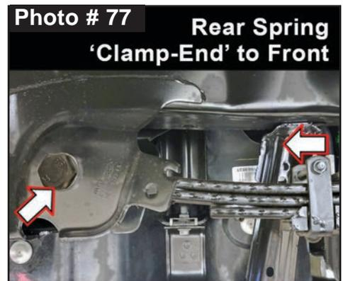
**Note:** 'Clamp-End' of Skyjacker leaf spring mounts to front frame mount. (Photo # 77)
