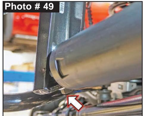
38. **6" Lift:** Remove OEM pitman arm nut from OEM steering gear using a 46mm socket \ wrench.
