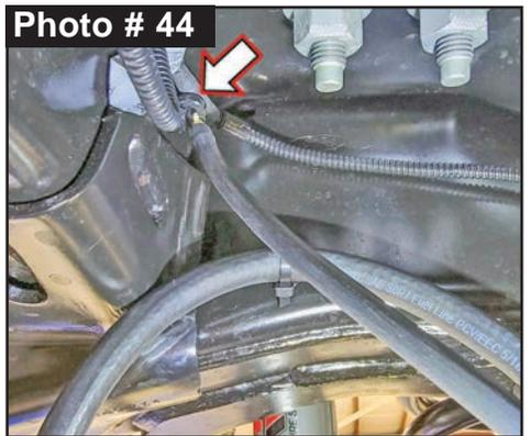
Replace with supplied # VT53224 5/32" x 24" Vacuum Tube. **Note:** Trim hose to needed length.
