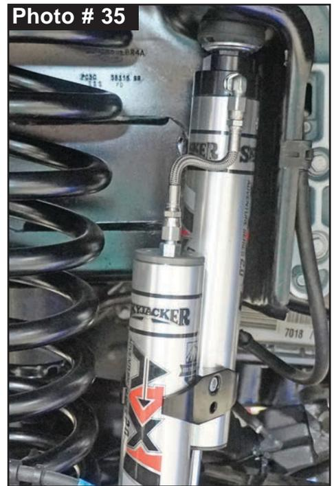
28. **Note:** Skyjacker Brake Line Extension Brackets Are Side Specific.
