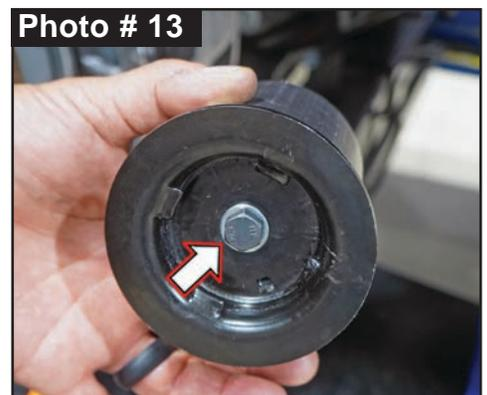
13. Install Bump Stop Spacer with OEM bump stop cup to frame mount using a 13mm socket \ wrench. (Photo # 14) Torque 23 ft-lbs.
