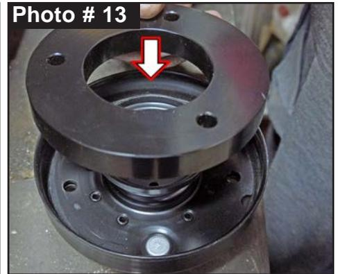
18. Install Skyjacker # F920MS-1 Aluminum Preload Strut Spacer in-between OEM upper strut mount & OEM coil spring isolator. (See Photo # 13)
