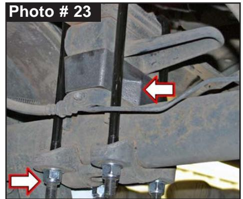
7. Install Skyjacker 9/16" U-Bolts over OEM top plate\leaf springs down into OEM u-bolt plate. Install supplied 9/16" Nylon Insert Nuts using a 7/8" socket\wrench. (See Photo # 23)
