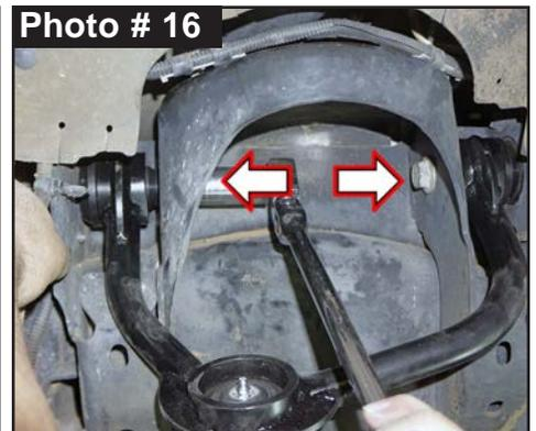
23. **Note:** Skyjacker\OEM strut assembly will install 180 Degrees from OEM orientation.
