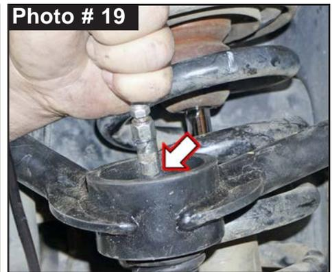
26. Grease Skyjacker UCA ball joint using a grease gun.
