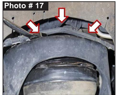
24. Install Skyjacker\OEM strut assembly into lower strut mount at OEM LCA with OEM hardware.
