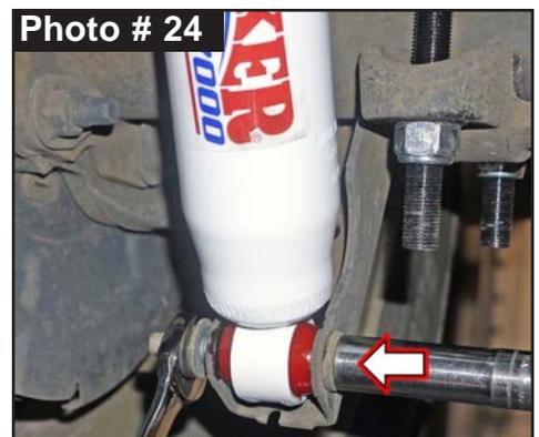
9. Locate Skyjacker ADX rear shock. Loosely assemble two (2) supplied reservoir clamps with two (2) supplied hex head bolts using a 5/32" Hex Key socket. Position clamp into place around shock body & reservoir cylinder. Secure, but **Do Not Completely Tighten** at this time.
