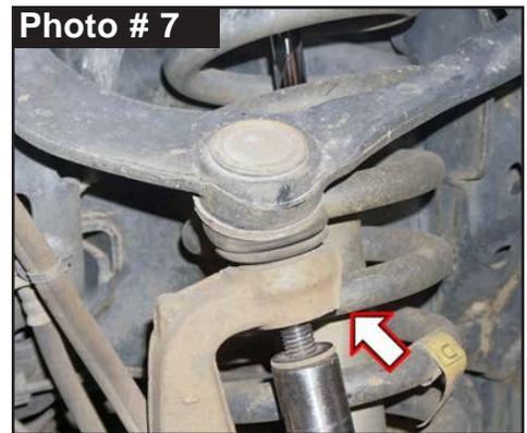
12. While supporting OEM Lower Control Arm (LCA), remove OEM CV-shaft from OEM steering knuckle. **Note:** Do Not Overextend CV Axle Shaft.
