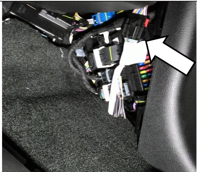
Plug in the 2017-2022 BD High Idle wiring harness to this connector.
