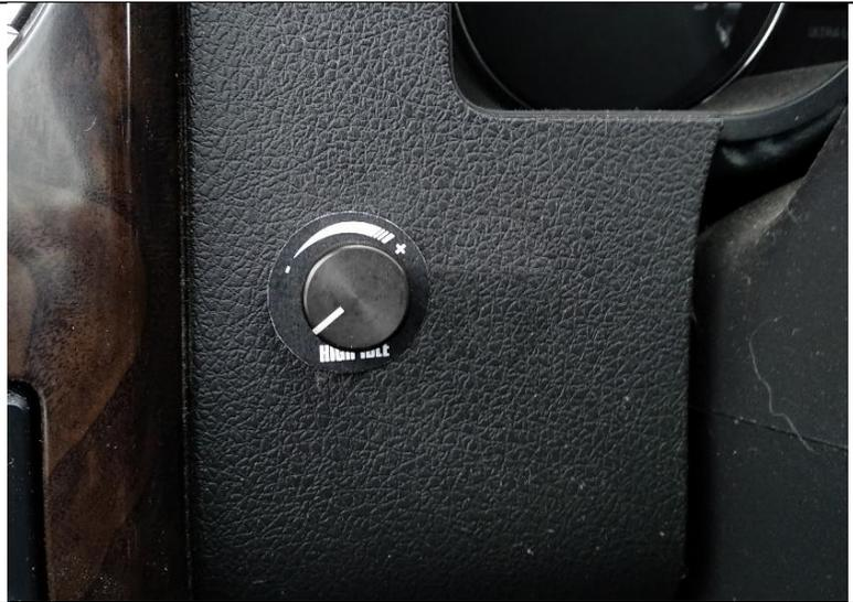
If mounting in the knee bolster, be aware of the reinforcement plate behind the bolster which will limit the available spaces to mount the switch.
