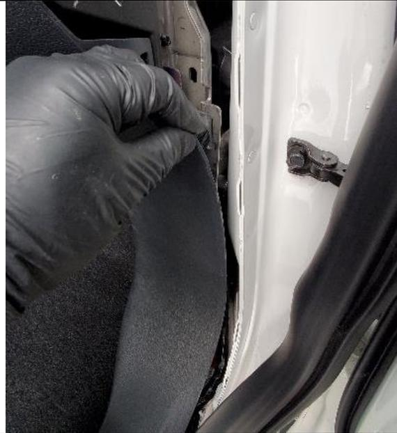
On some 2023+ trucks the up-fitter pigtail is accessible after removing the kick panel. The pigtail can be identified by the bundle of wire terminals taped together and connected to a grey connector.
