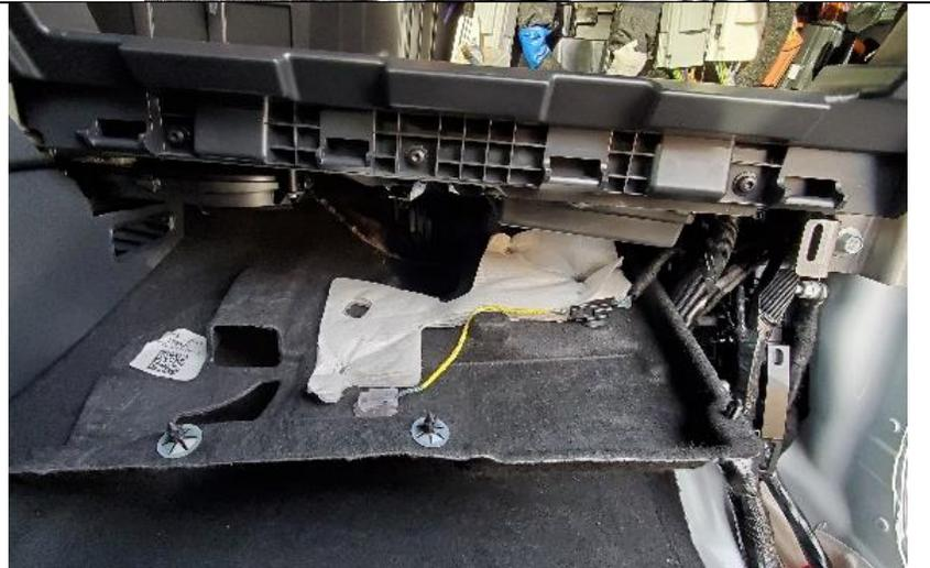
The pigtail location has been found to vary from truck to truck. Shown here is the most hidden and inaccessible spot. The metal bracket that held the plastic panels can be used as a reference point.
