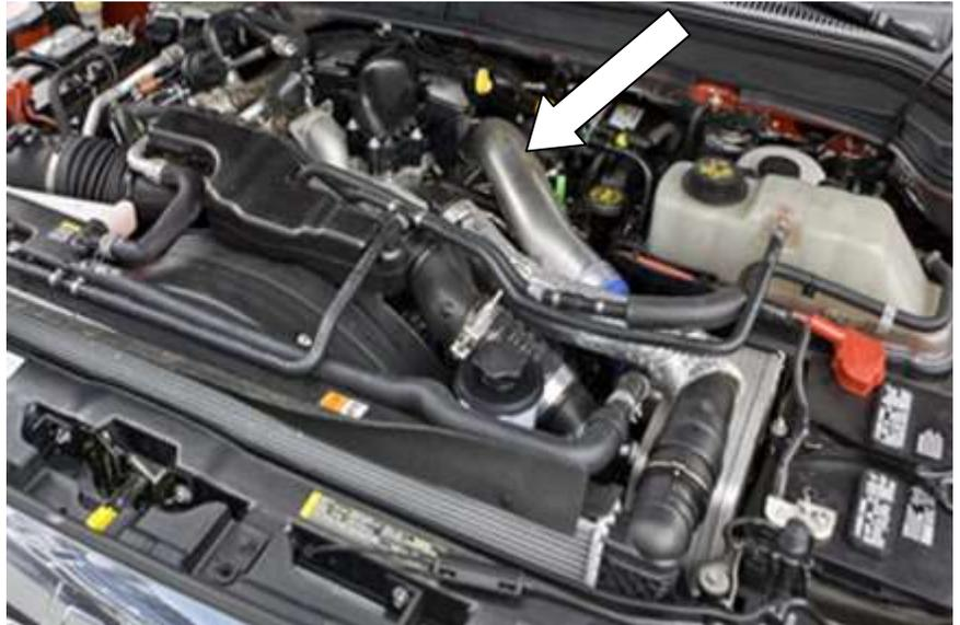
3. Once the pipe is removed from the truck, you can make your first cut at 4 1/2" from the factory pipe benders grip start on the C.A.C. side.
