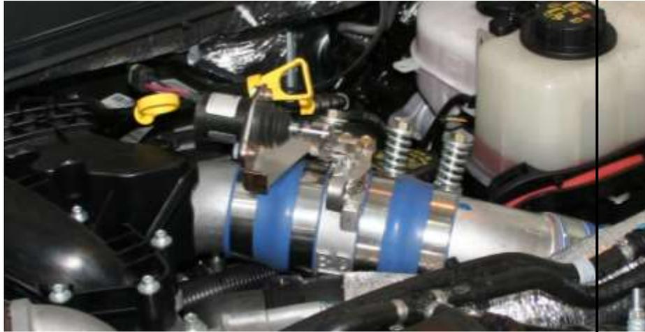
12. Lay out supplied harness over top of the driver's side of the engine.
