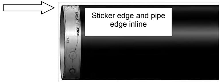
5. With the sticker in place use a center punch and then use a  $\text{Ø}1/8$ " drill bit and drill a hole in the center of the holes marked "For 3Ø".
