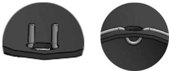
8. Now slip the small side of the boot over the bead ring and pipe assembly.
