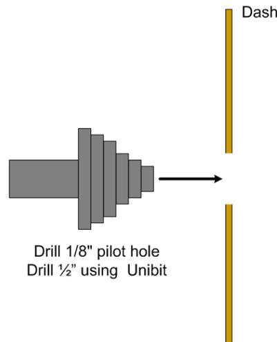
13. Once you have the mounting hole drilled, crimp the switch connectors to the switch wires and install the correct switch wires to the correct switch terminals then insert the switch into the dash from the backside.
