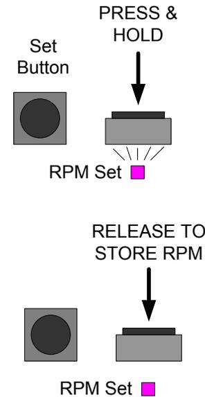
You should see the RPM signal flash proportionally to engine RPM.
