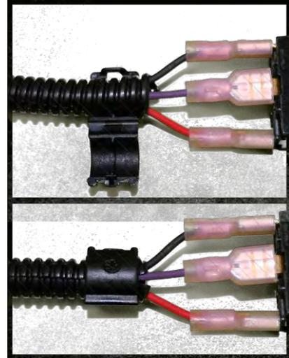
**INSTALLATION without OVER SPEED ELECTRONICS (1036730-M & 1036731-M)**
