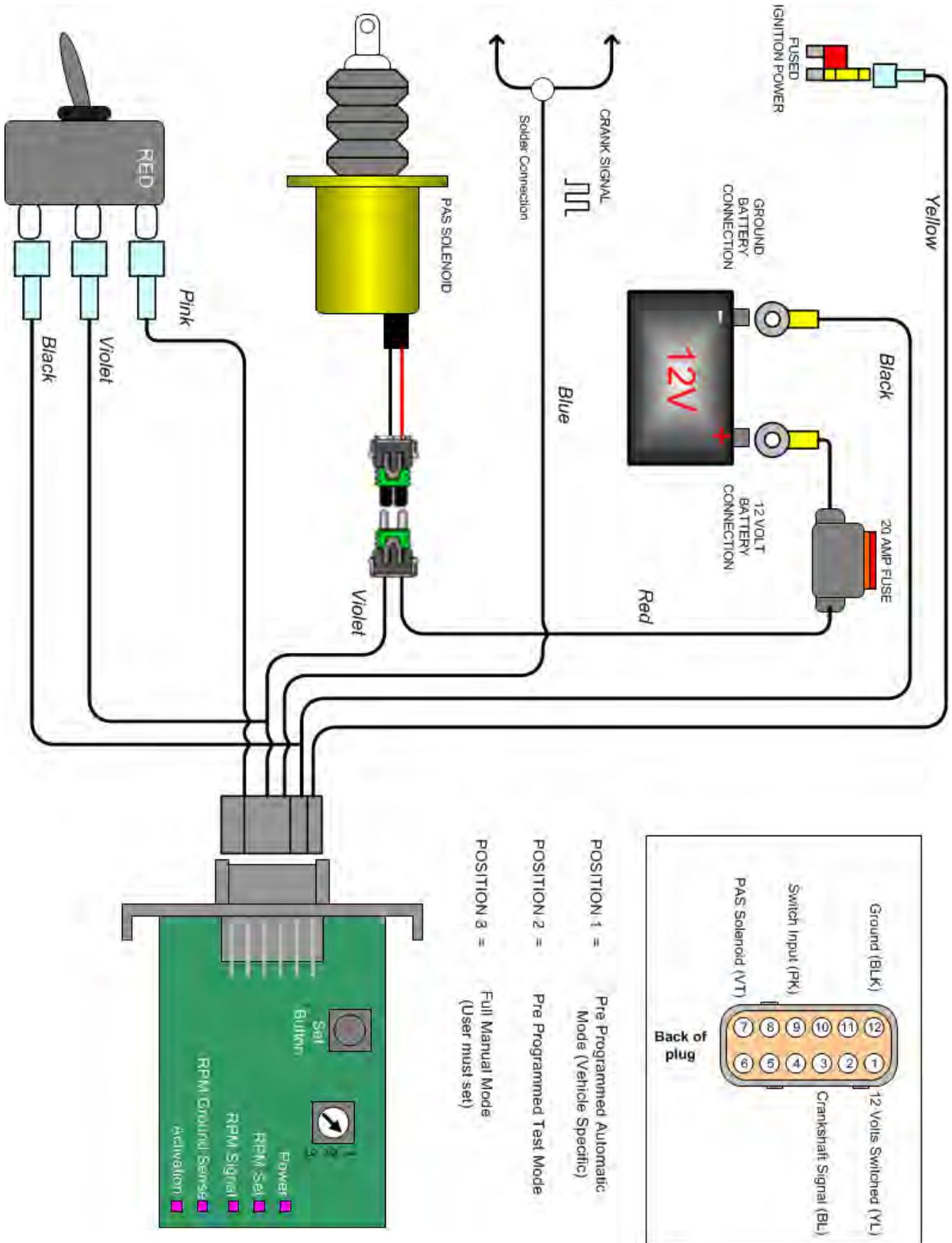
**WIRING DIAGRAM without OVER SPEED ELECTRONICS (1036730-M & 1036731-M)**
