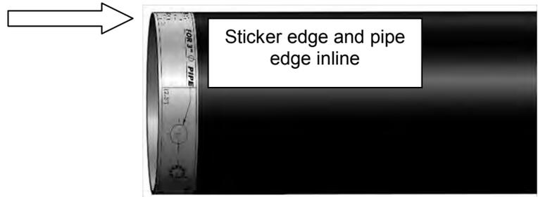
5. With the sticker in place use a center punch and then use a  $\varnothing 1/8$ " drill bit and drill a hole in the center of the holes marked for the 2.5" or 3" pipe size.
