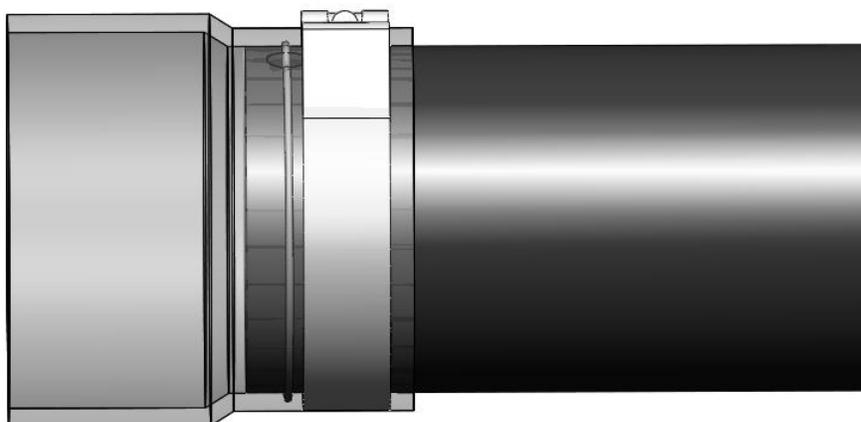
9. You can now install the valve into the open 3.5" section of the boot. Use the 1407030 (0350) spring clamp to secure this connection.
