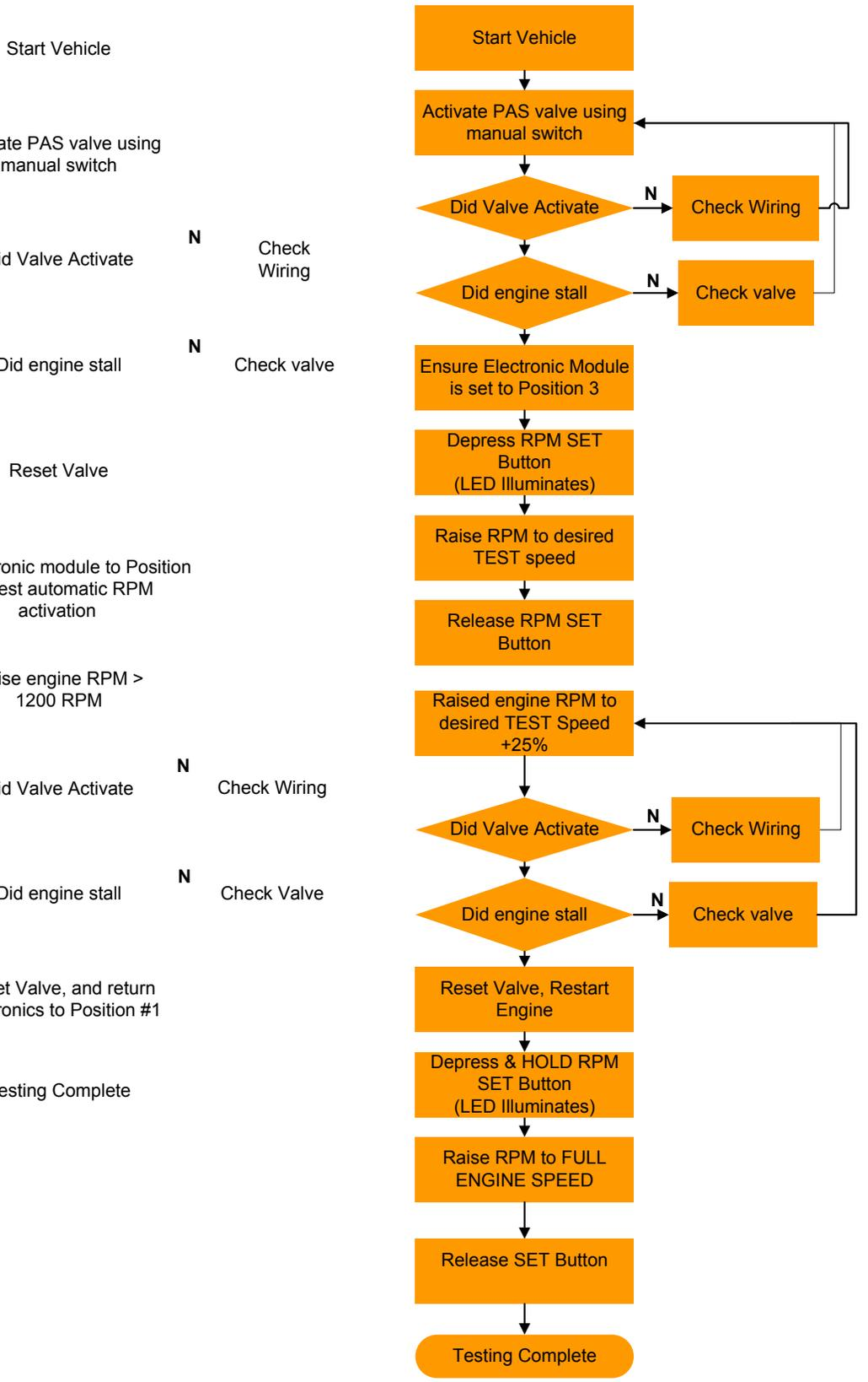
**TESTING FLOW CHART without OVER SPEED ELECTRONICS (1036730-M & 731-M)**
