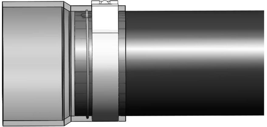
9. You can now install the valve into the open 3.5" section of the boot. Use the 1407030 (0350) spring clamp to secure this connection.
