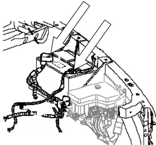
19. For the last connection you will need to locate the vehicles ignition power. This will power the automatic over speed control box LED switch. Note that the unit can still be activated manually with the switch at any time.
