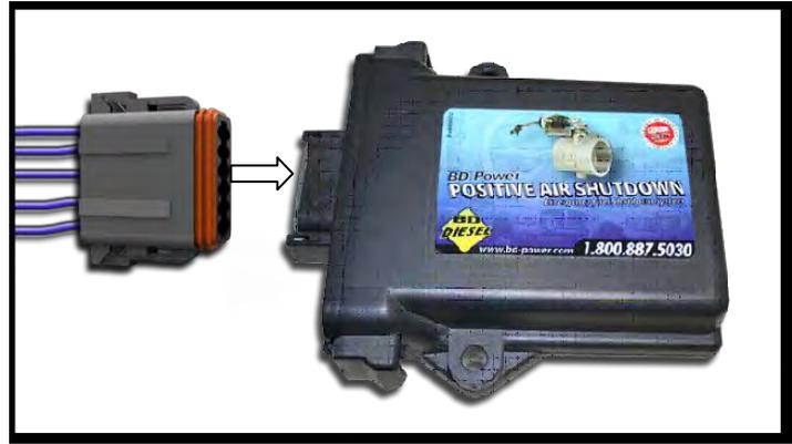
13. Locate the PAS valve solenoid connector. Then butt connect the violet wires from the switch & solenoid to the violet wire from the module and heat shrink the connection.
