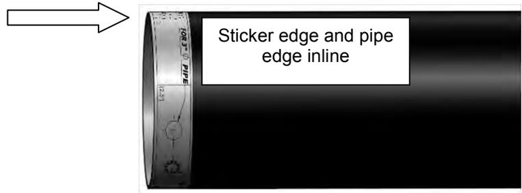
5. With the sticker in place use a center punch and then use a  $\text{Ø}1/8''$  drill bit and drill a hole in the center of the holes marked for the 3.5 or 4" pipe size.
