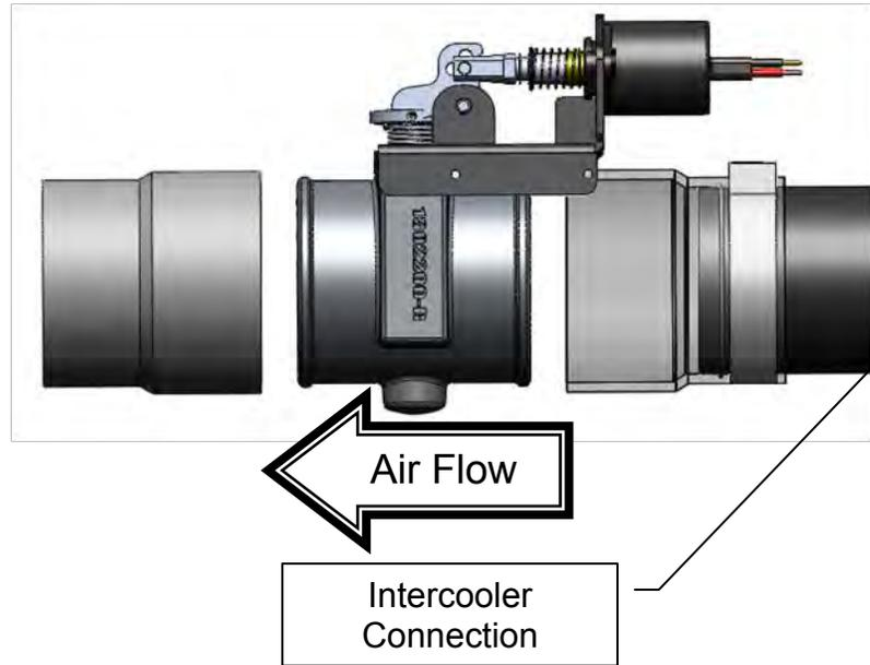
11. Locate the weather pack connector on the solenoid and connect the wiring harness solenoid plug and lay out the harness over the engine bay.
