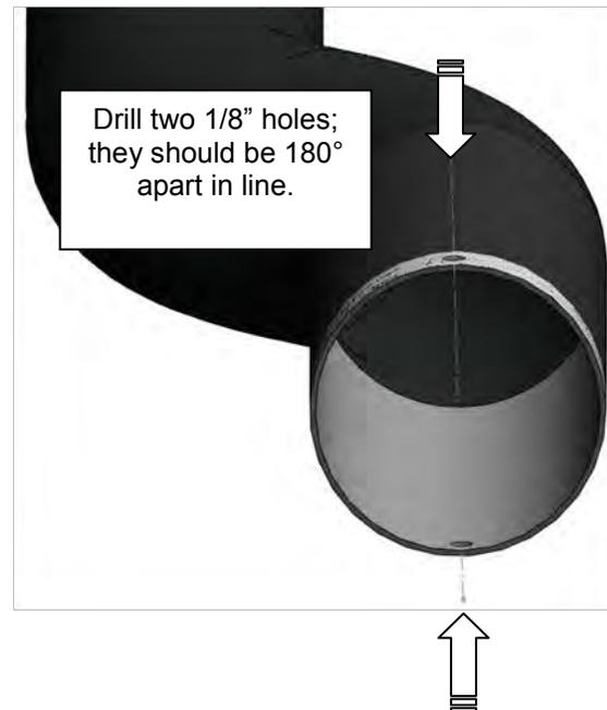
6. Once the pilot holes are drilled you will need to drill a  $\text{Ø}11/32$ " hole through the pilot holes.
