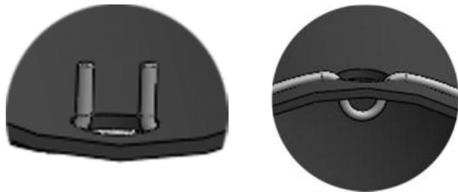
8. Now slip the supplied clamp (0378 for a 3.5" pipe) or (0411 for a 4" pipe) over the bead ring onto pipe and slide the small side (for a 3.5") or any side (for a 4") of the boot over the bead ring and pipe assembly.
