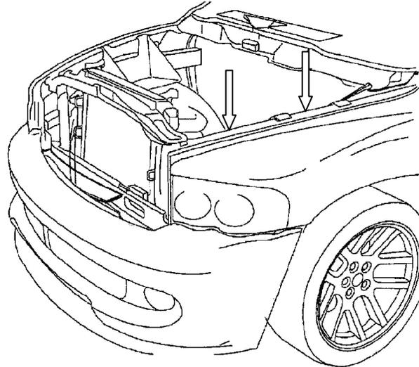
12. Next plug in the harness to the module and lay out the harness over the engine bay and run the violet wire to the solenoid.
