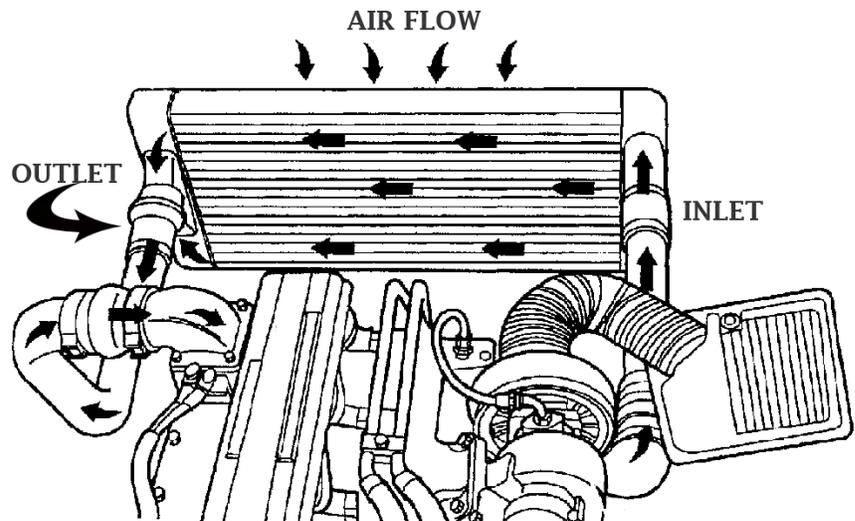
3. You may need to cut down your CAC outlet pipe before installing the bead ring to allow for the installation of the positive air shutoff valve.
