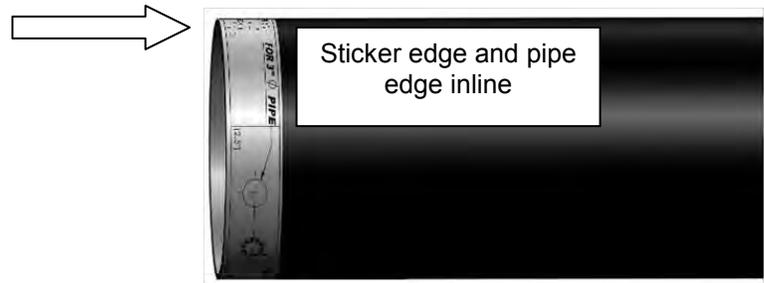
5. With the sticker in place use a center punch and then use a  $\text{\O}1/8$ " drill bit and drill a hole in the center of the holes marked 3.5 or 4" pipe size.
