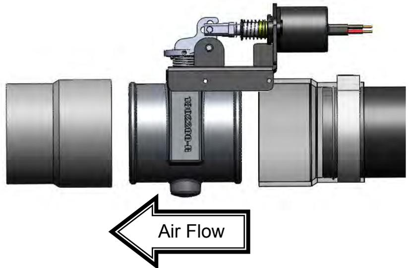
10. Finally, reinstall the PAS and pipe assembly back into the truck; securing the intercooler end first. Then using the supplied clamp secure the intake end.
