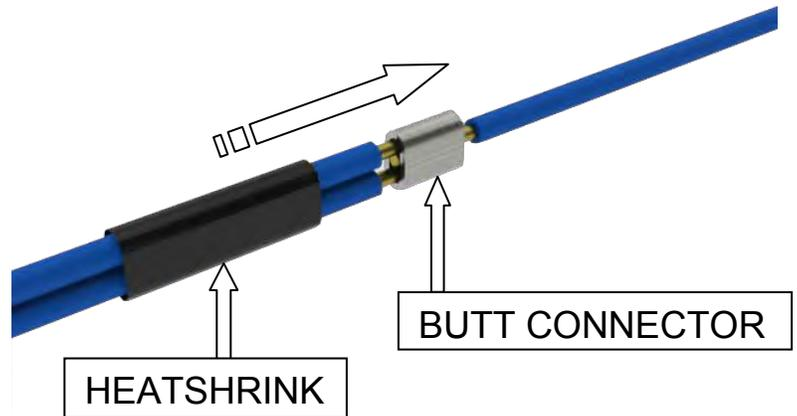
14. Under the hood locate the ECM / PCM / or Crankshaft wire. Being that the RPM signal is critical you will need to solder the connection.
