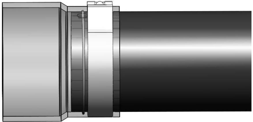
9. You can now install the valve into the assembly. Use the 0411 spring clamp to secure this connection.
