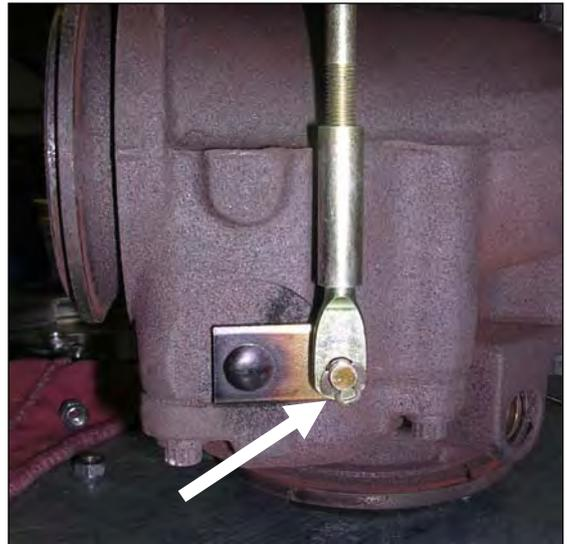
Use a 7/16" socket and remove the two mounting nuts that secure the wastegate to the housing.
