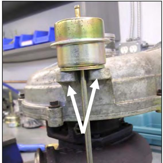
Install the BD adjustable wastegate. Use the two new locking nuts that are supplied in the kit to secure the wastegate diaphragm to the compressor housing. Apply air to the wastegate port to stroke the actuator. Once stroked, you should be able to slide the rod end over the wastegate lever shaft. Re-install the cir-clip.
