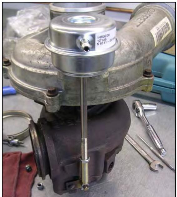
The waste gate is preset to allow 25psi of boost pressure. One full turn of the rod clockwise (shortening the rod) will increase boost pressure by 5psi. One half turn will increase boost pressure by 2.5psi.
