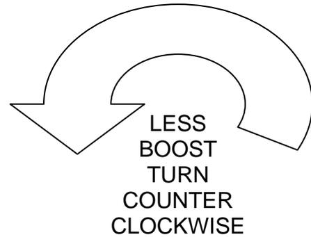
To increase the boost pressure you will have sufficient energy to drive the turbo faster. Once you have turned the rod to the desired position, re-install the circlip and lock the jam nut.
