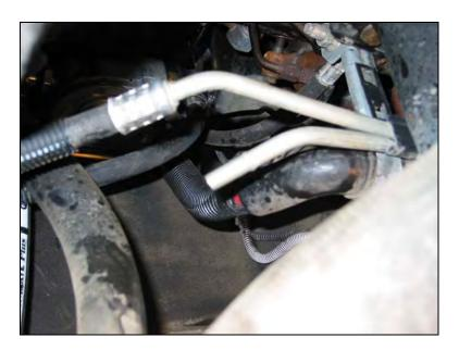
Push a hose clamp over the outlet hose from the filter and attach the hose to the straight fitting just installed on the steel line, cutting any excess hose. Tighten the hose clamp.
