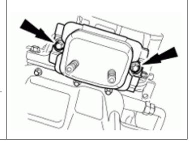
bolt and 9. Loosen the disconnect the transmission vehicle harness connector.
