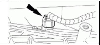
20. Connect the transmission vehicle harness connector.
