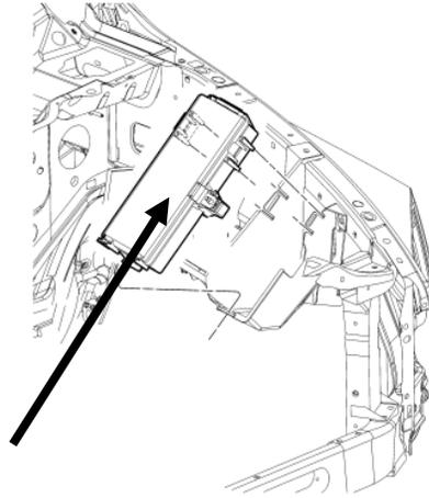
At the very bottom of the IPM, locate the appropriate connector (C10). Locate **Pin 18 OR/RD** and use the Red T-Tap to tap this wire. Use the supplied wire to route this connection back to the CDT "Trans Pump" output.
