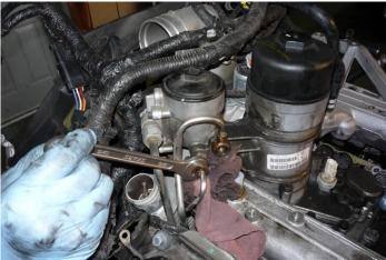
Reinstall the oil filter and EGR valve, service both as required.
