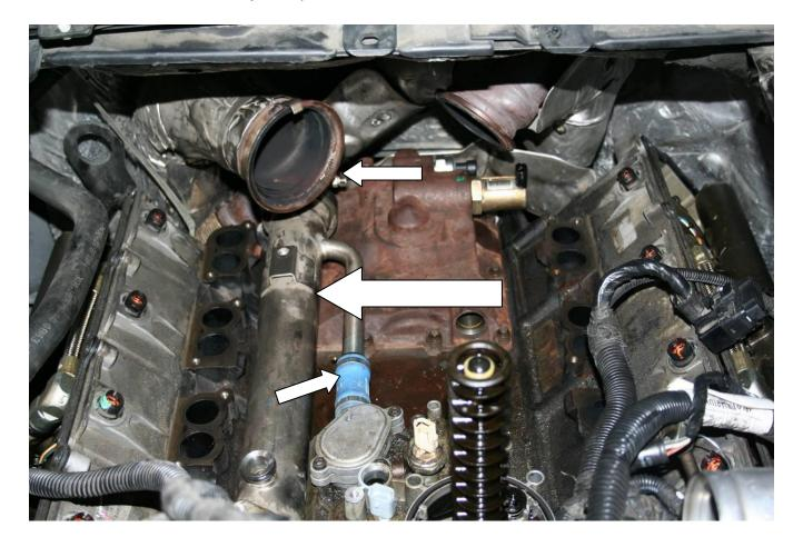
Remove the EGR cooler by disconnecting the clamp at the exhaust feed pipe then remove the coolant hose by first twisting about 90° and sliding back along the cooler tube.
