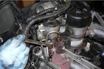
Disconnect the fuel filter wiring connectors and fuel lines then remove fuel filter housing.
