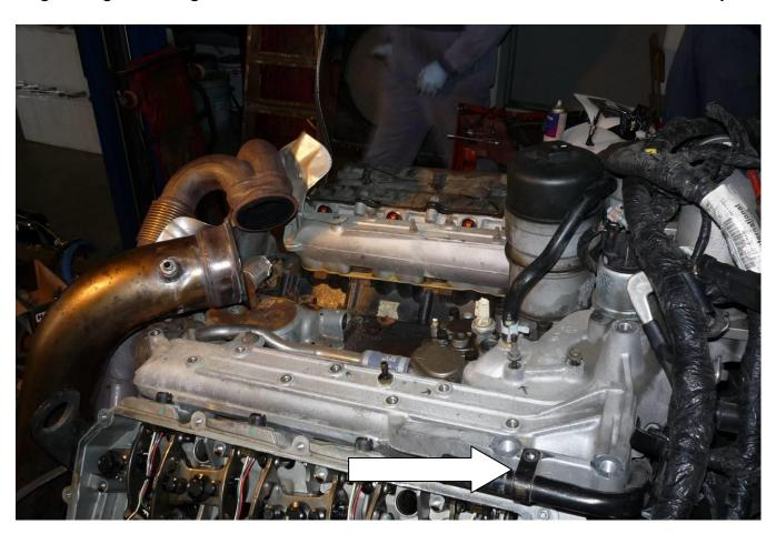
9. Reinstall the oil drain pipe & turbo pedestal mount using four (4) 10mm mounting holts
