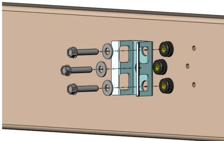
2. Insert the three rubber isolators into the support bracket. Use some water to aid in lubricating the isolators as they slide into the bracket.
