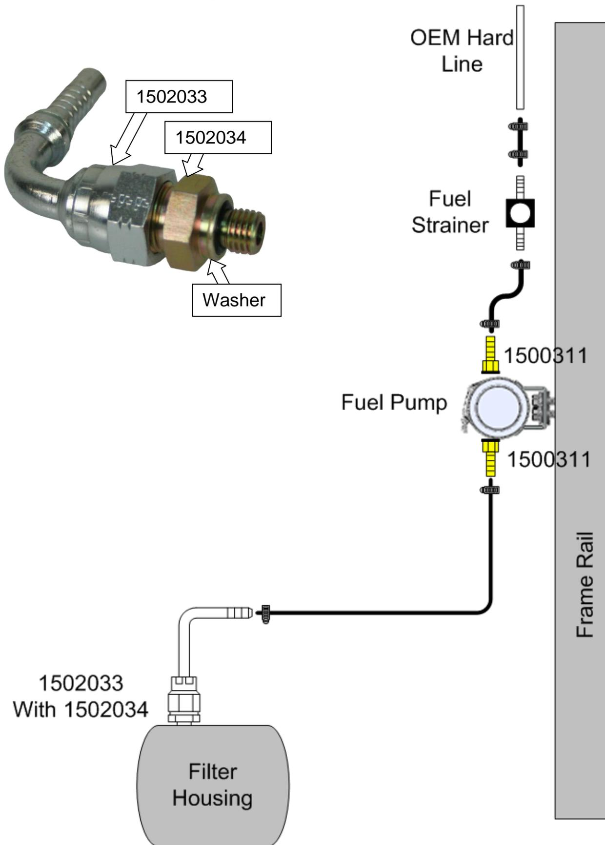
6. Remove the stock lift pump from the side of the engine along with fuel line back to where the line was cut along the frame rail and up to the fuel filter bowl. At the fuel bowl the banjo bolt will need to be removed as well since it is being replaced.
