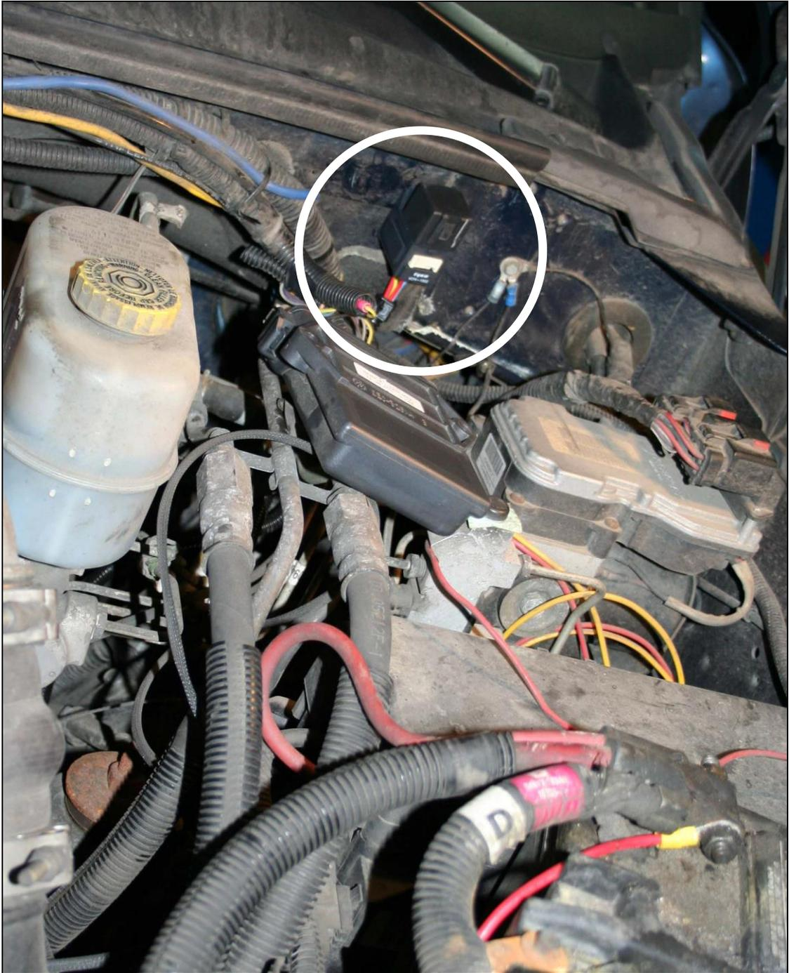
9. Wiring should be attached with the use of supplied tie wraps so that the wiring will be away from contacting hot surfaces and/or moving components. Once the wiring is attached and everything is in place the positive and negative terminals can be attached to the battery.
