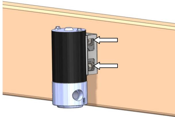
With both clamps inserted, place the pump into place and align the inlet and outlet parallel to the frame. The **inlet** should be pointed towards the fuel tank.
