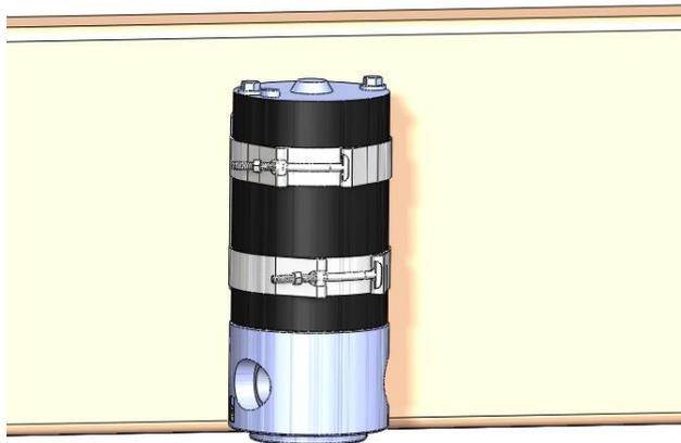
4. Insert the ORB-Barb fittings into the inlet and outlet of the pump. Do not over tighten as they use an O-ring for sealing.
