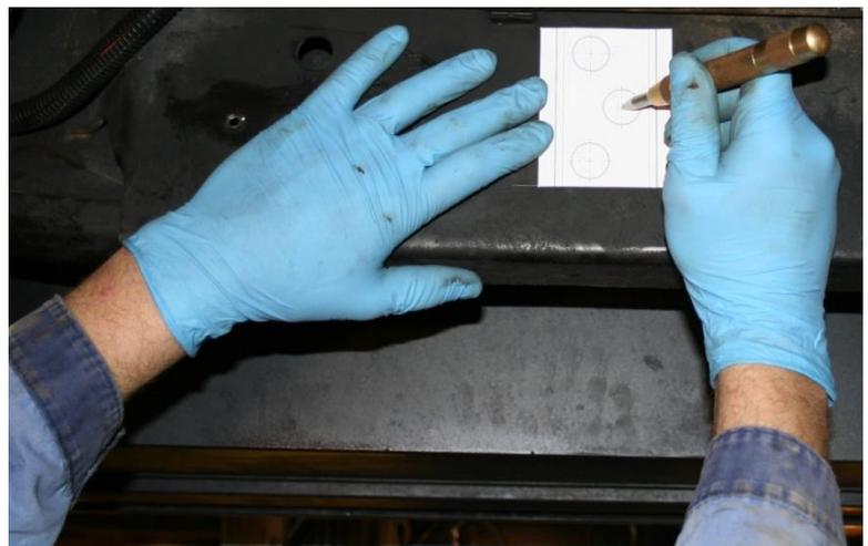
1. Center punch the three holes, remove drill template and drill a pilot hole to 1/8". Then re-drill to 11/32".
