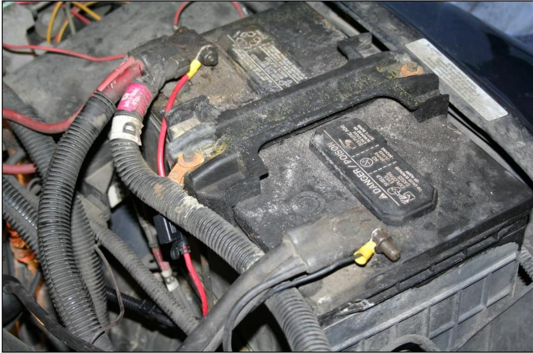
10. Make sure that all fuel lines, wiring harness' are fixed in place well.
