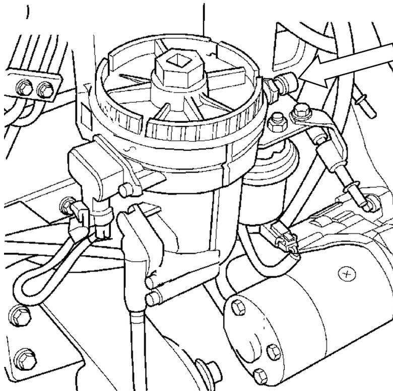
7. Thread the JICM adapter (1502033) into the fuel filter bowl and tighten first. Do not over-torque as this is an o-ring seal. Then thread on the JICF adapter (1502034) position the barbed end and tighten.
