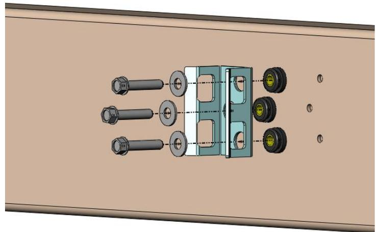
10. Insert the three rubber isolators into the support bracket. Use some water to aid in lubricating the isolators as they slide into the bracket.
