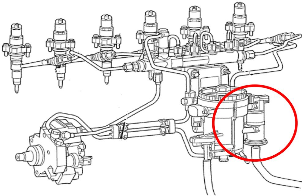
4. Install the brass 90° NPT to barb fitting into the supplied aluminum pump bypass bracket. The brass elbow should be orientated so that the barbed end points down or oriented 90° to the mounting holes. You will need to use Teflon sealant to seal the threads.
