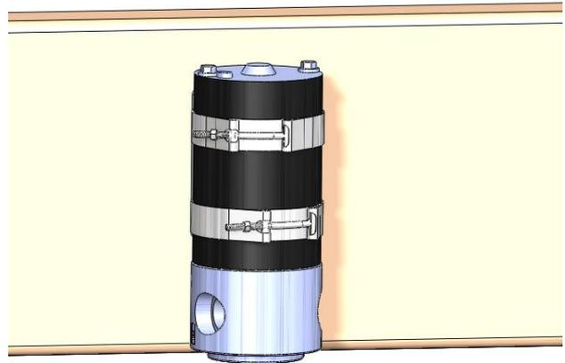
Tighten the clamps around the motor body, rather than the aluminum pump head. Torque nuts to **80 in-lbs.**
