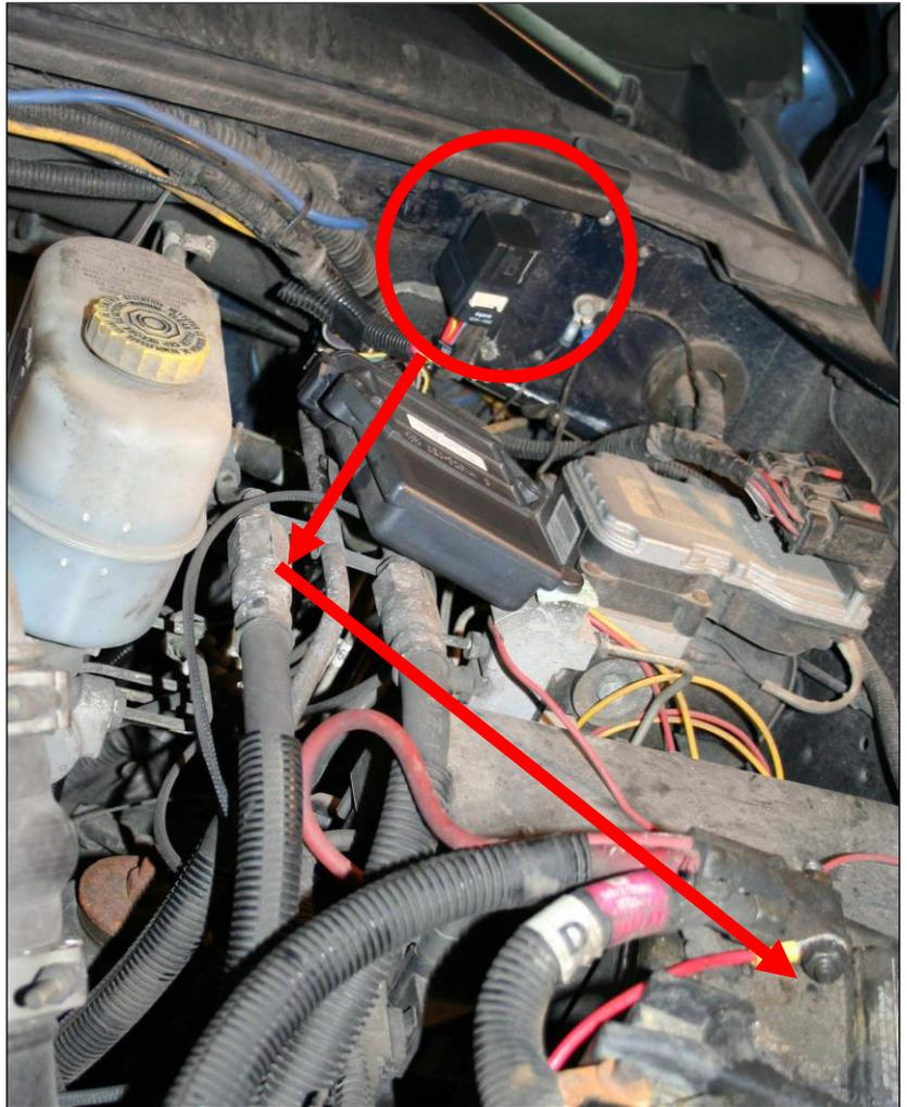
18. Wiring should be attached with the use of supplied tie wraps so that the wiring will be away from contacting hot surfaces and/or moving components. Once the wiring is attached and everything is in place the positive and negative terminals can be attached to the battery.
