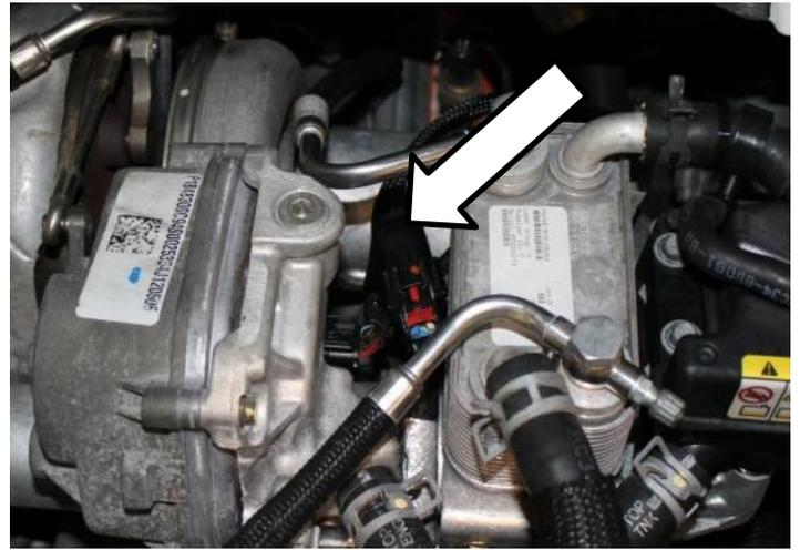
9. Secure wiring harness away from moving parts and heat sources using the supplied cable ties.
