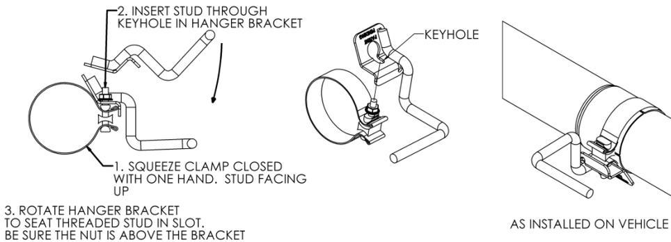
4. Place the previously assembled **Hang Tight™ Hanger** onto the end of the **Over-Axle Pipe**, leaving the clamp loose. Install the **Hang Tight™ Hanger** into the factory rubber isolators.
