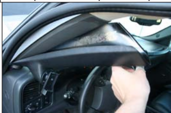
Line up A-Pillars & push into place
