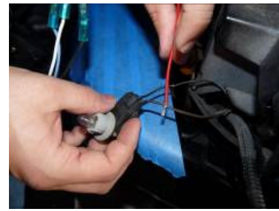
Step 12: Get the new Anzo light and splice the red (+) wire to the brown wire on the parking light.
