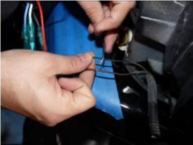
Step 13: Splice the black (-) wire into the black wire of the parking light to light up the leds.
