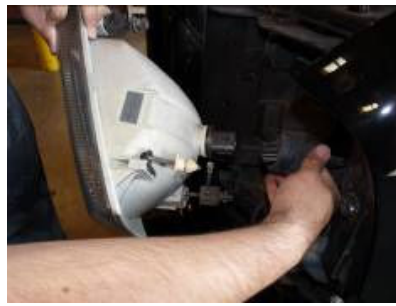
Step 11: Unclip the head light wire harness.
