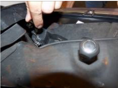
Step 16: Use the supplied locking clip on the top corner to hold in the head light.
