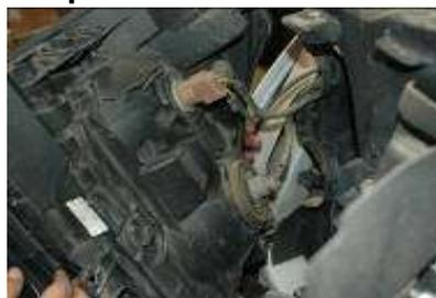
Carefully pull out the OEM headlight and expose the parking and turn signal power sources.
