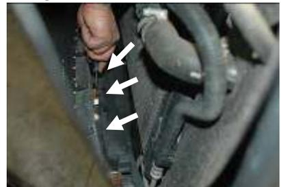
Using the phillips screw driver push down and unlock the three clips located on the bottom of the grille.
