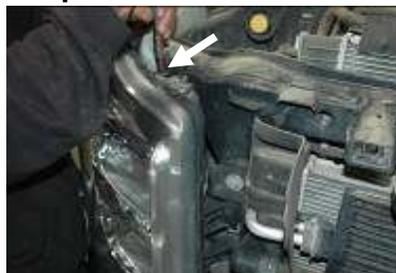
Remove the 10mm bolt located on the top of the OEM headlight housing.
