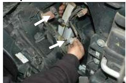
Remove the OEM headlight by disconnecting the parking and turn signal power sources.
