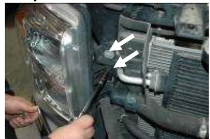
Remove the two 10mm bolts located on the side of the OEM headlight housing.
