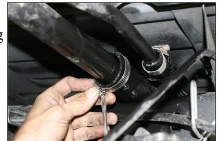
**Helpful Hints: If more space is required to access the top of the fuel tank, loosen the strap nuts to the end of the stud. This will gain you about 3” more working room.**
