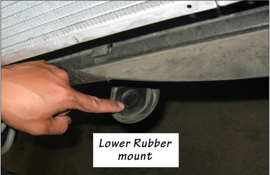
**Figure 9** Connecting Fuel Cooler Radiator to Banks Techni-Cooler
