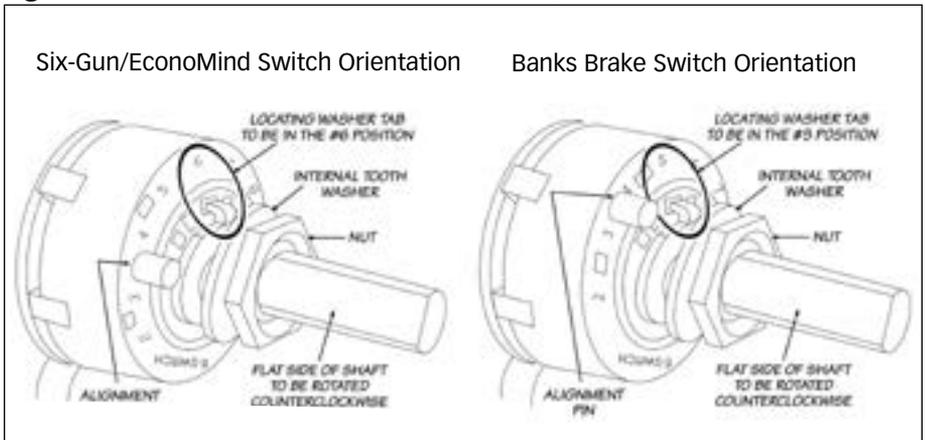
**Figure 28:** Finished installation of the Six-Gun/EconoMind/Brake switches on 2003-04 vehicle
