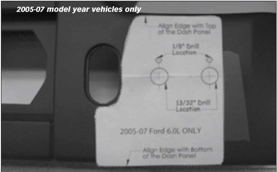
**Figure 26:** 05-07 Dash panel trimming
