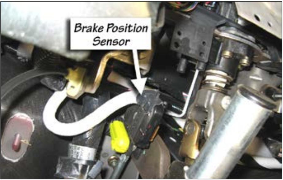
**16.** Locate the Brake Position Switch intercept connectors on the Banks Brake Wire Harness. Connect the female connector on the Brake Position Switch intercept connectors to the factory black brake position switch connector. Connect the male connector on the Brake Position Switch intercept Connectors to the factory female brake position connector that was disconnected.
