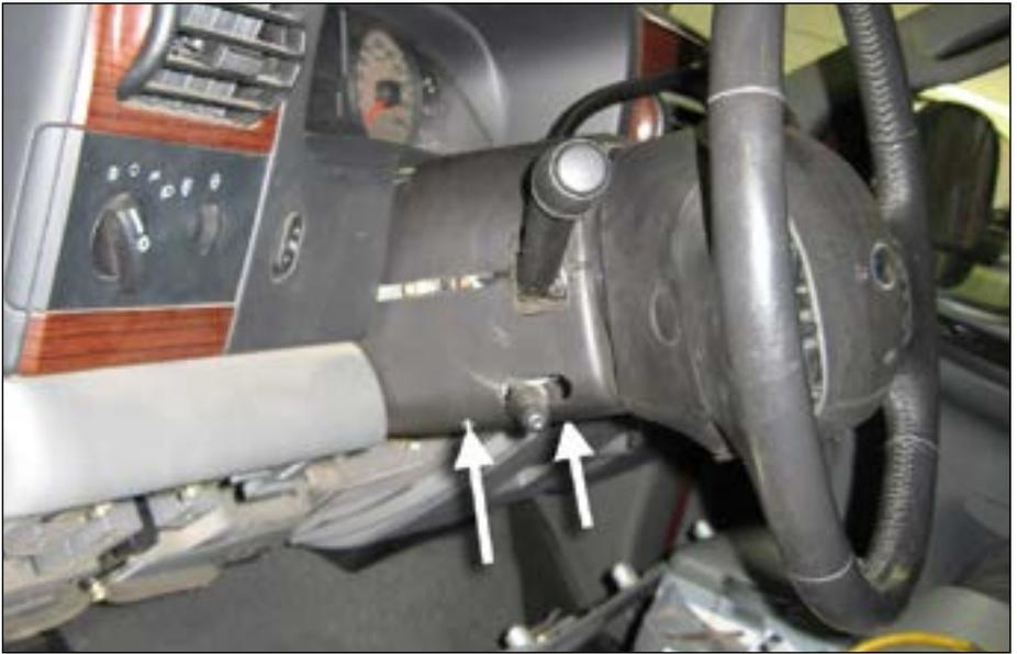
**Figure 20** Remove Plastic Ignition Key Guide
