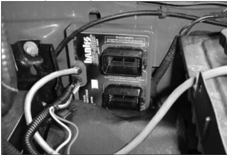
**Figure 4:** Six-Gun/EconoMind installed on the fuse box on 2005-07 model-year vehicles
