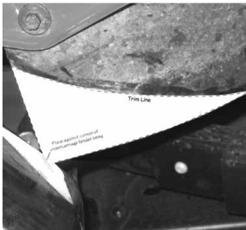
Placement of template on passenger side rear undercarriage lining.
