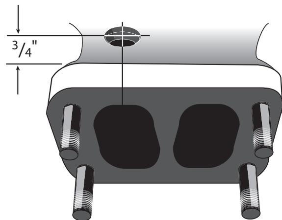
Tap the drilled hole with a ¼" NPT pipe tap. Check the thread depth as you tap by periodically removing the tap and screwing the sensor fitting into the tapped hole. The sensor should thread in three to three-and-a-half turns hand-tight.
