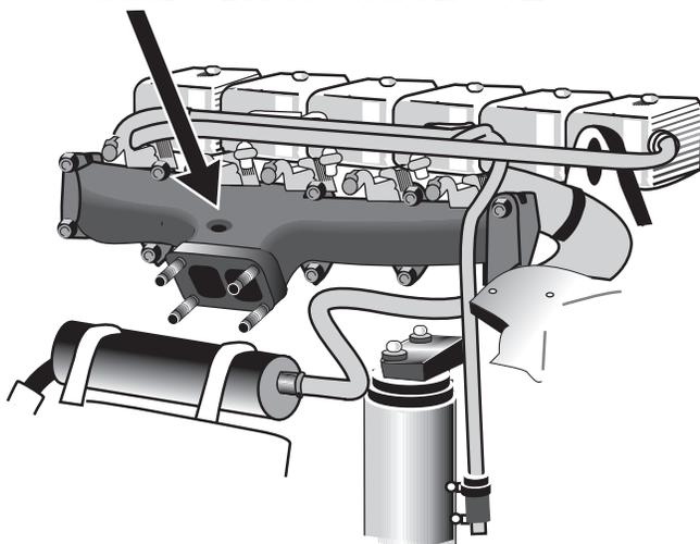
*LOCATE PORT  $\frac{3}{4}$  INCH BEHIND FLANGE CENTERED OVER REAR EXHAUST MANIFOLD PASSAGE*
