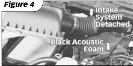
**5.** Remove the black acoustic foam covering the passenger side camshaftcover and EGR cooler outlet pipe. See **Figure 4**.
